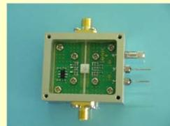
The Ku-band 3-stage MMIC low noise amplifier (NF=1.7dB) and the module
