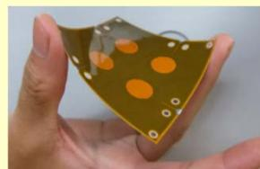
The 2x2 antenna array with a flexible print substrate
